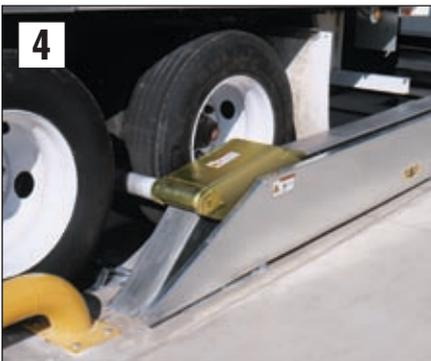
4 The locking arm automatically sizes the tyre and rises to its full height against the tyre.
