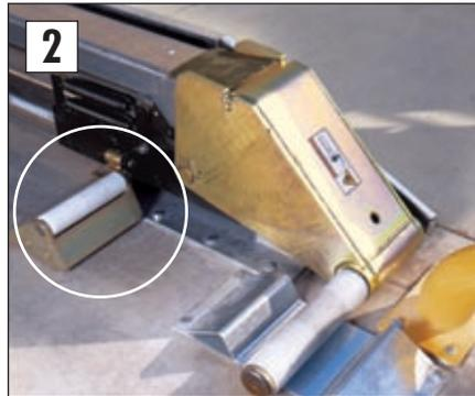
2 The rearmost tyre contacts the restraint's trigger device...
